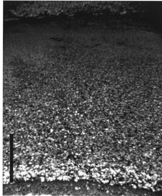
Figure 6. High-magnification photomicrograph of a single varve from piston core 95DON-05. Normal grading from fine sand to clay-sized grains is discernible, as is well-sorted nature of silt grains comprising the main body of the varve. Scale bar = 1 mm.
